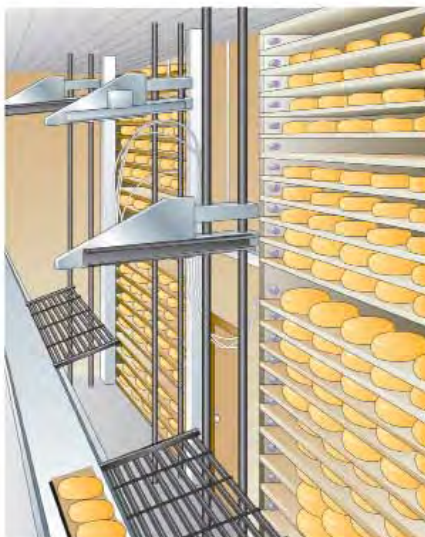
Figure 38: Mechanised cheese storage. Humidified air is blown through the plastic nozzles at each layer of cheese.
