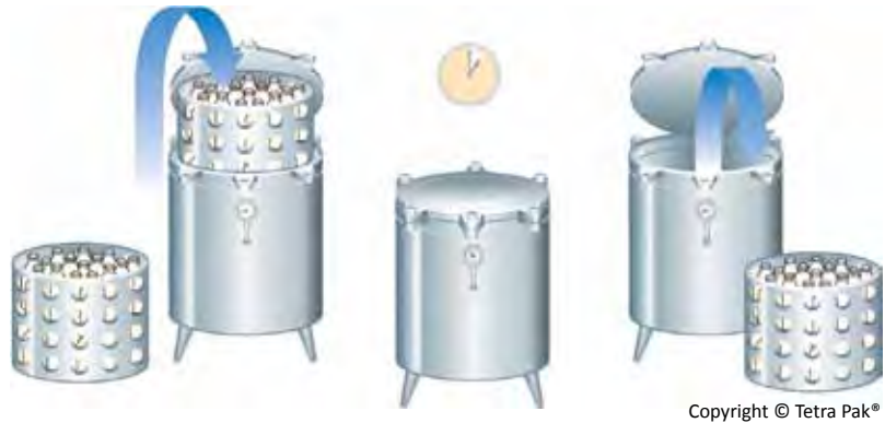
Figure 22: Batch processing in a static pressure vessel (autoclave)
