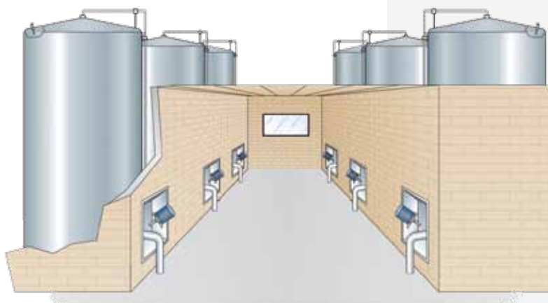
Figure 6.9.1: Layout of outdoor silo tanks with their manholes in alcoves in the walls of a covered control station
